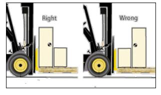
Load as close to the front wheels as possible to minimize the distance from the front wheels to the load center. Load the heaviest part toward the mast (shown at left).
