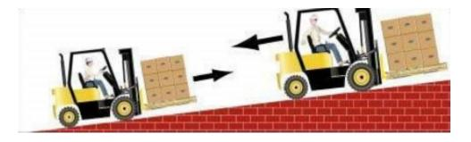
When driving on an incline or decline *without a load*, always operate the PIT with the forks pointing downhill (shown below).
