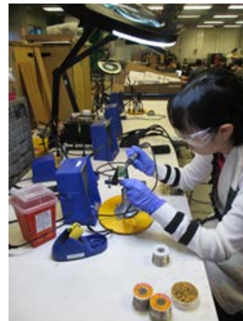
Designated soldering area with fume extractors at each station
