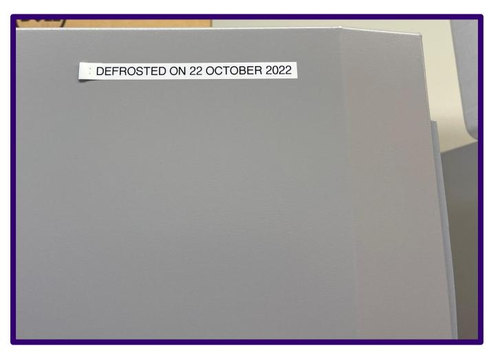
Manufacturers recommend defrosting freezers at least once a year or more frequently if the freezer is prone to ice build-up. For labs that have more than just a couple of freezers, it can be challenging to keep track of defrost schedules.
