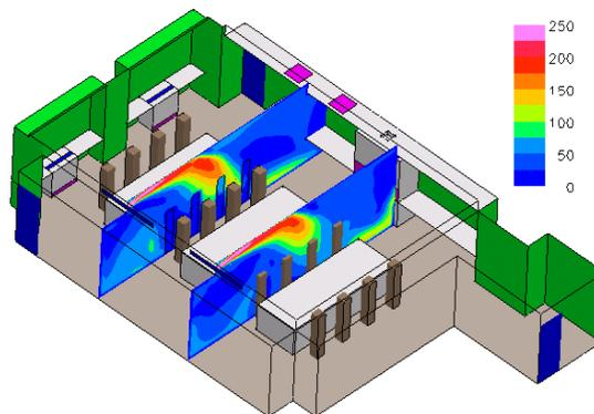
**Figure 3 - Corrected Momentum to Match Diffuser Throw Data**
