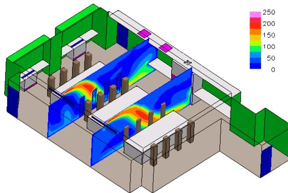
**Figure 2 - Incorrect Modeling of Supply Momentum**
