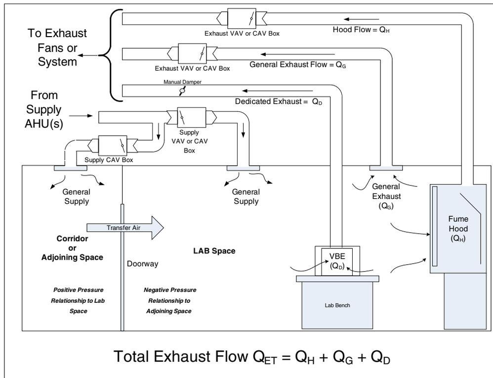
**Figure 2.** Lab Spaces may have multiple fume hoods, multiple general exhaust grilles, and multiple devices requiring dedicated exhaust. To calculate ACH based on exhaust for negatively pressurized labs, all exhaust sources must be included in the summation.
