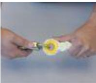
B) Thimbles: The thimble must be firmly seated in the eye of the splice, and the splice should have no loose or cut strands. The edges of the thimble must be free of sharp edges, distortion, or cracks.
